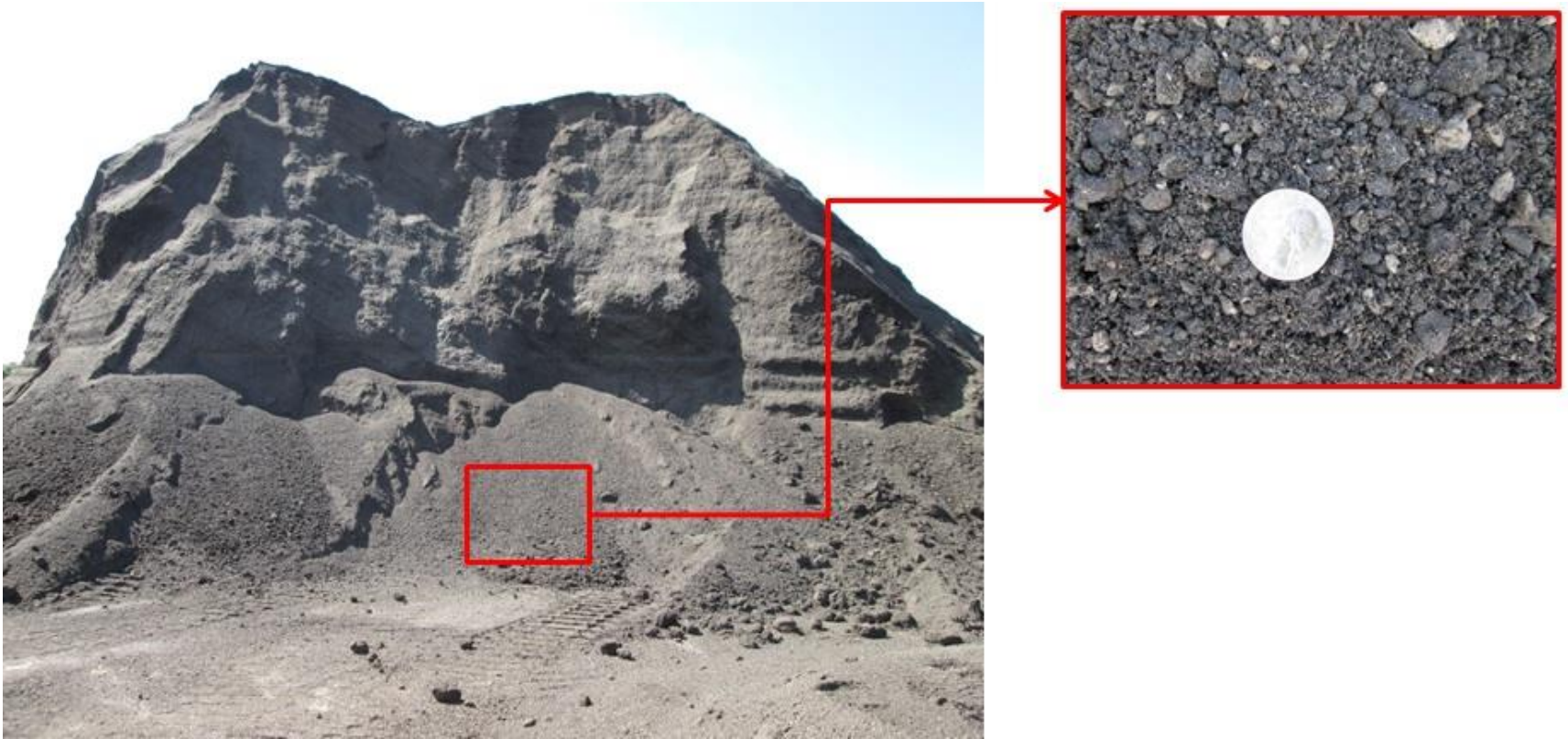
RAP stockpile (1/2" RAP Townline Pit – 52400-26)
