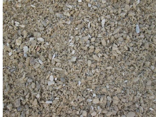
Washed Manufactured Sand (WMS)
